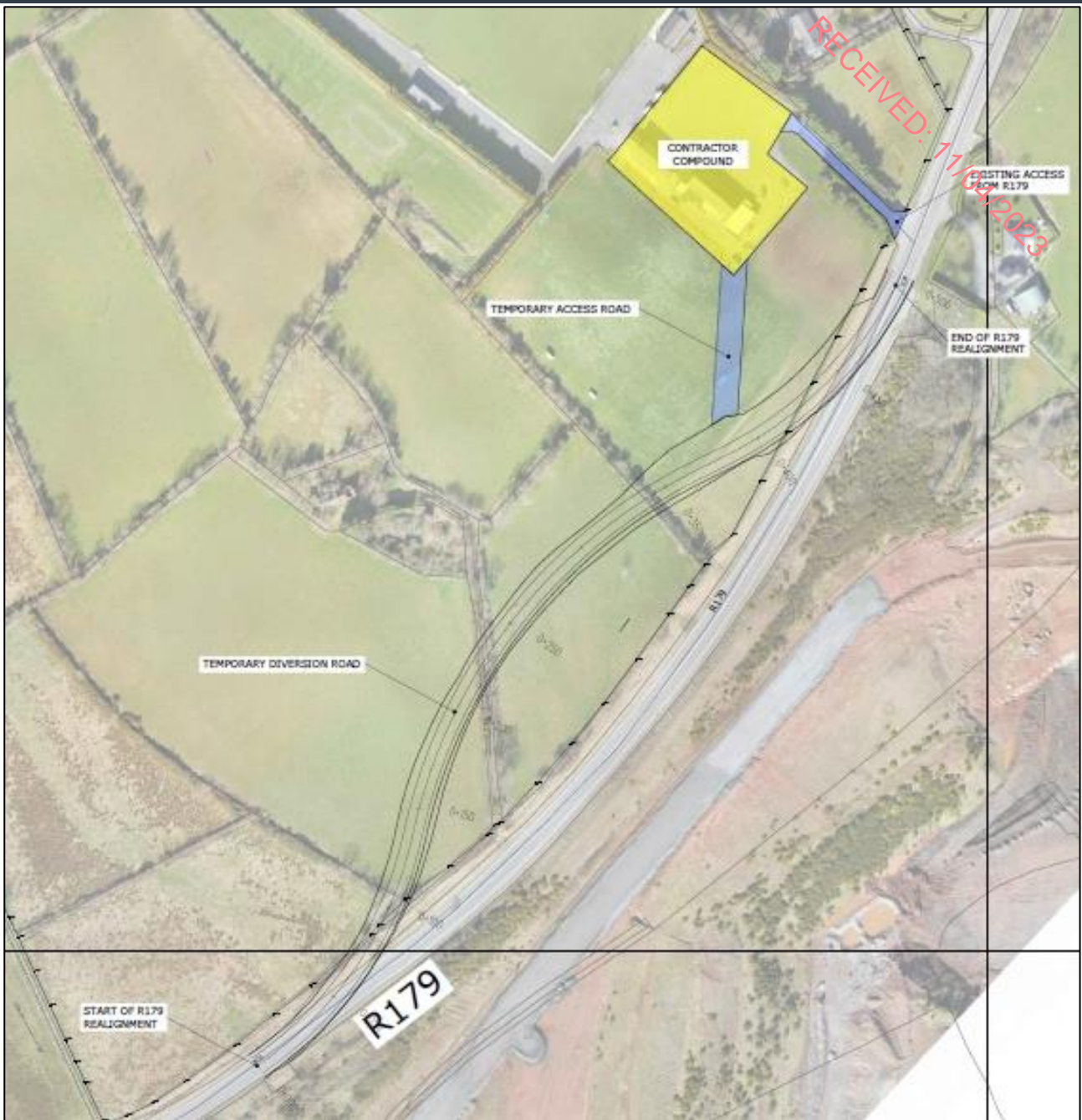
Figure 9: Construction Compound and Site Access for Temporary Diversion Road
