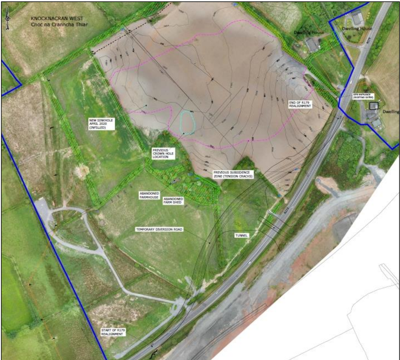
Figure 4: Plan showing extent of the Subsidence Event and the footprint of Temporary Diversion Road
