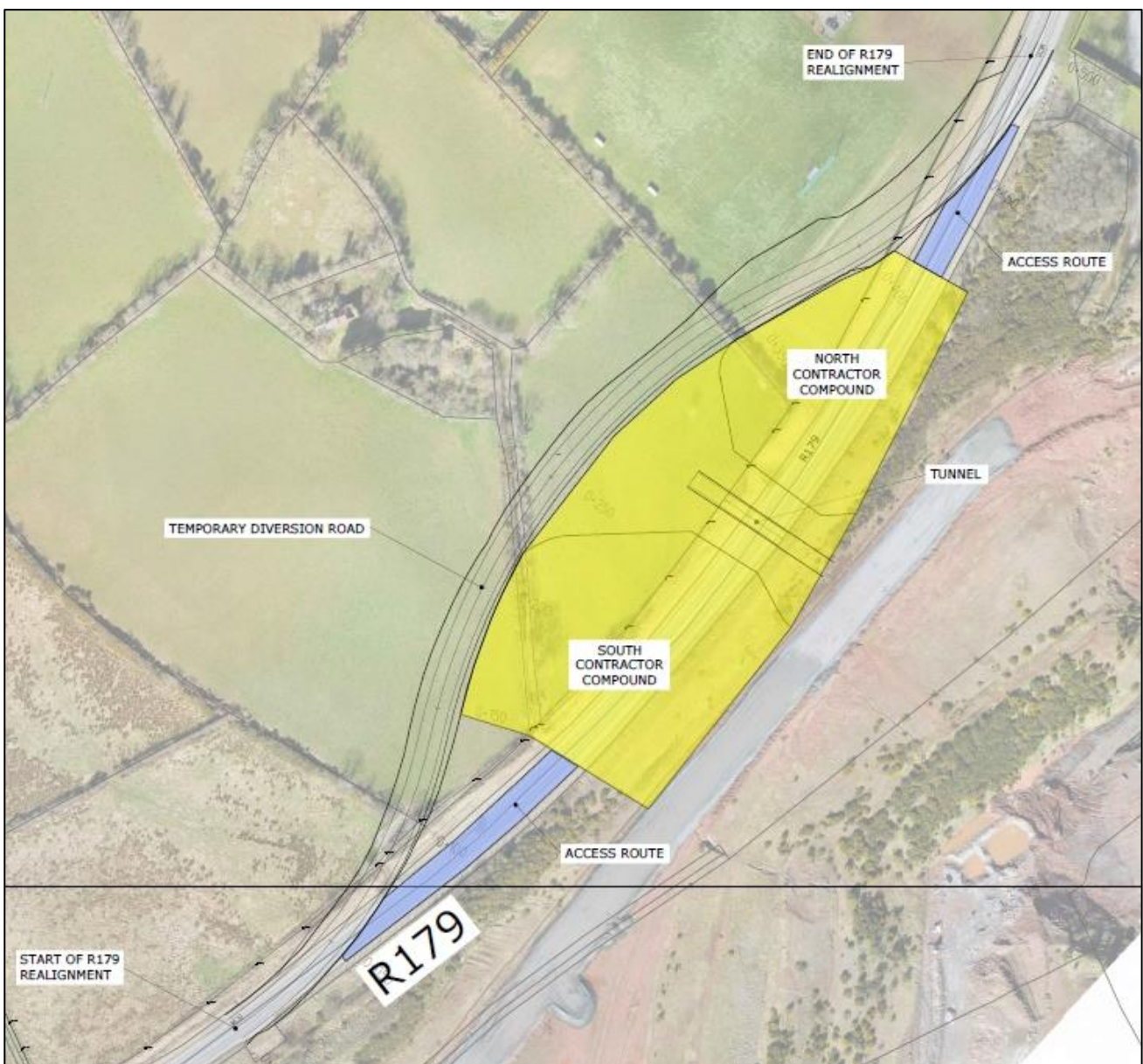
Figure 10: Construction Compound and Site Access for Cut-and-Cover Tunnel
